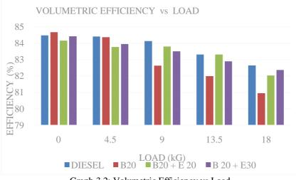
Graph 3.2: Volumetric Efficiency vs Load
