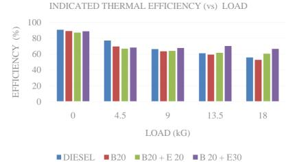
Graph 3.4: Indicated Thermal Efficiency vs Load
