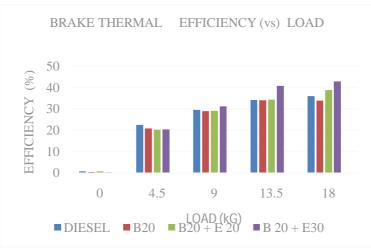
Graph 3.5: Brake Thermal Efficiency vs Load
